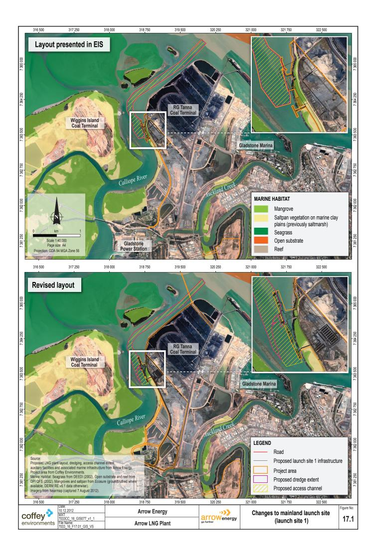
The updated model has provided more detailed information on changes in the frequency, duration and extent of exposure of the intertidal area following completion of dredging. The impacts of a reduction of extreme low tide levels and flow-on effects to the ecology of the river were not addressed in the EIS.
