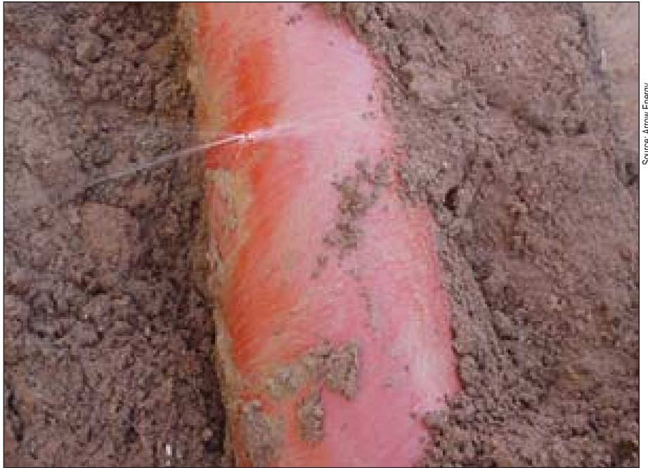
Plate 7.7 Leak detected in hydrostatic test of pipeline
