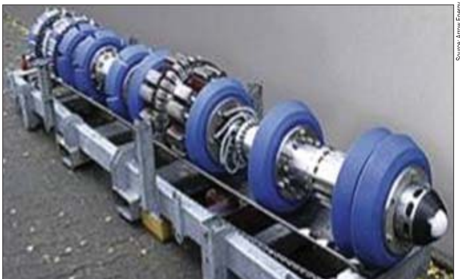
Plate 7.9 Typical intelligent pig
