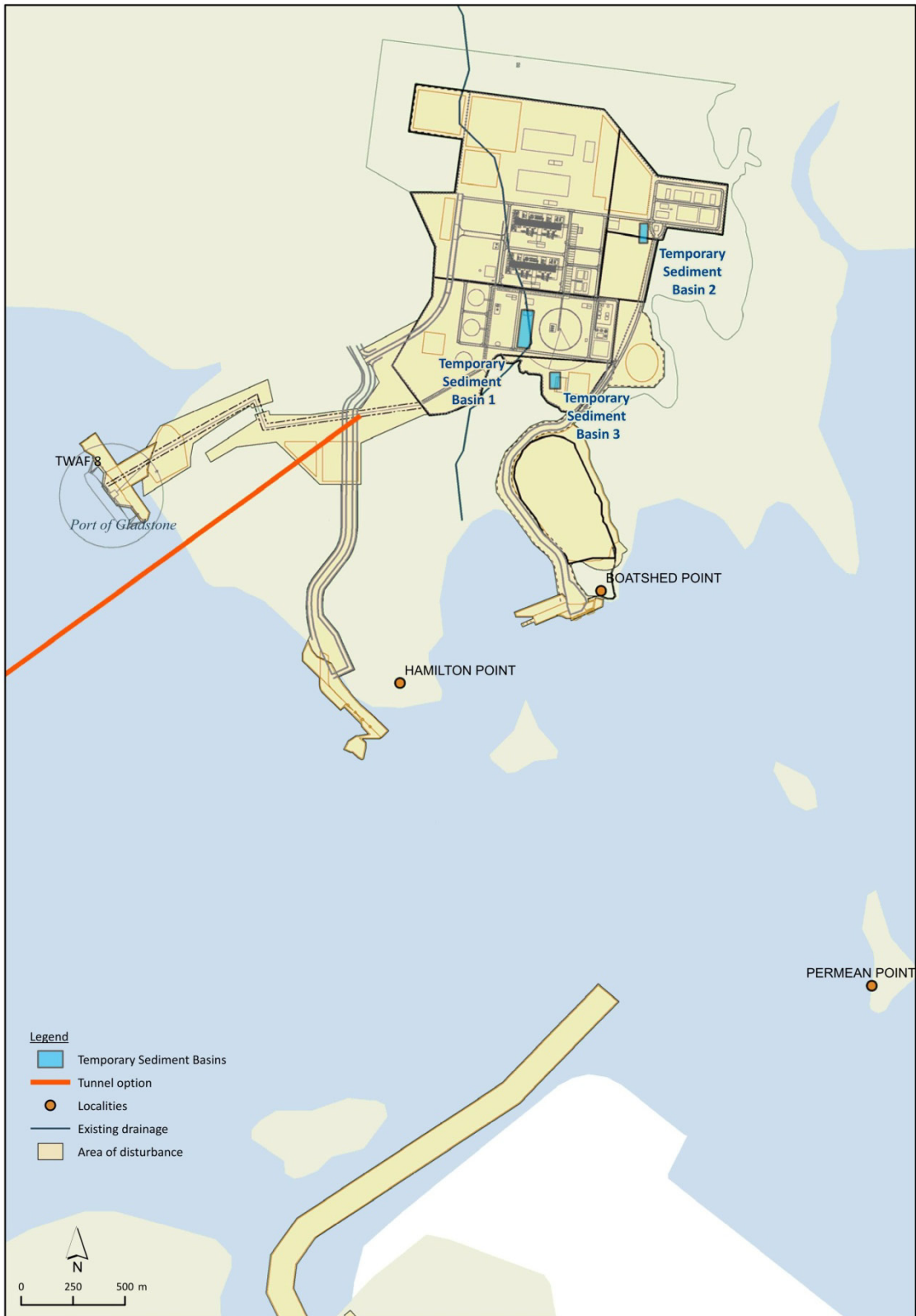
Figure 2. Proposed stormwater treatment system arrangement LNG plant (construction phase)
