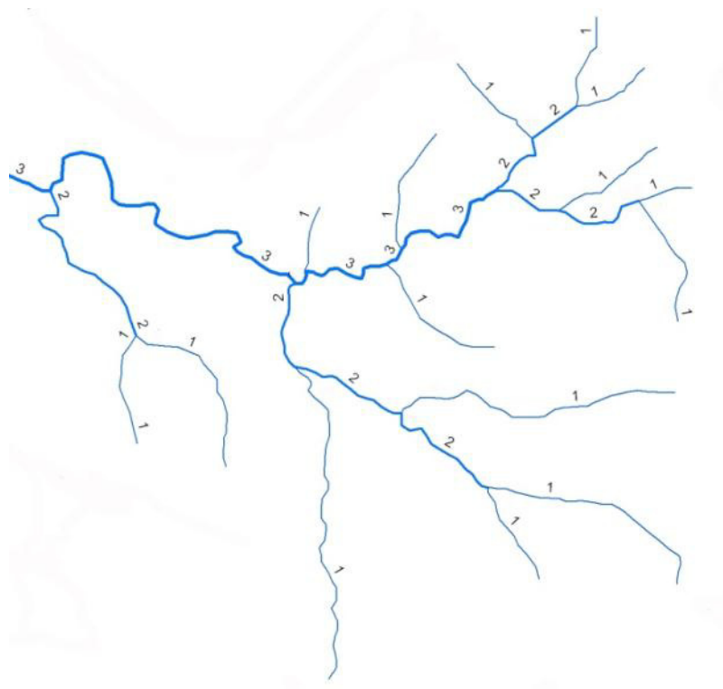
Figure 3-1. Strahler stream ordering
