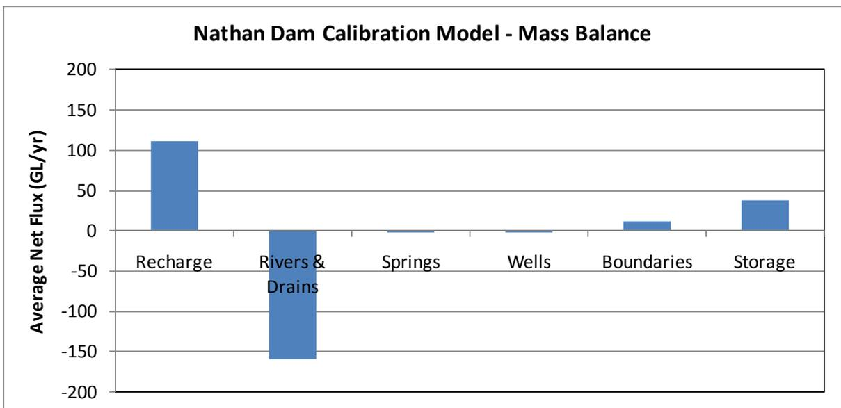
Figure 16 Average Net fluxes in the Nathan Dam Calibration Model (negative values indicate a net discharge)
