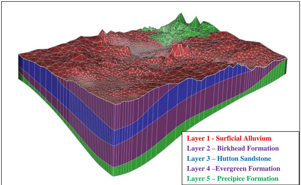
Figure 1 3D block diagram of the model layer structure
