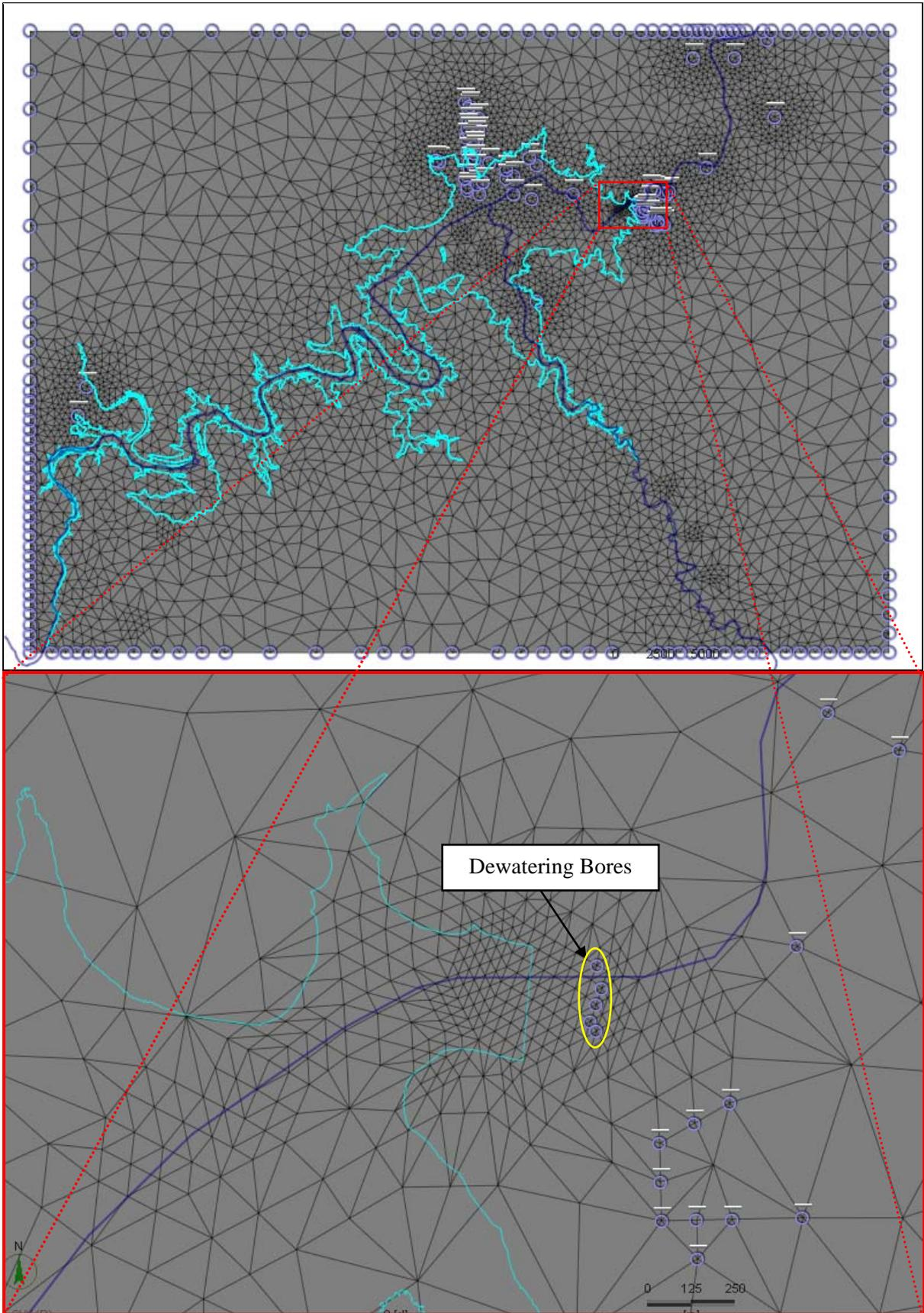
Figure 18 Refinement of the Feflow mesh for the dewatering scenario
