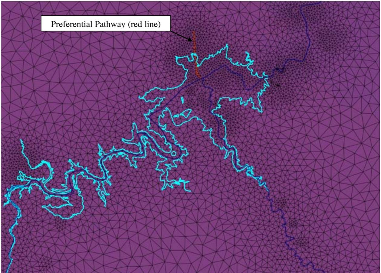
Figure 2 Location of a preferential pathway placed under the springs to the north of Glebe Weir.
