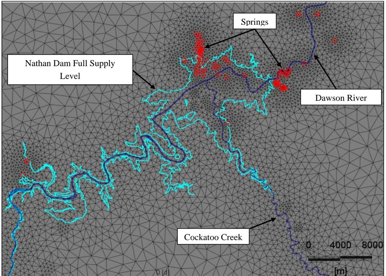
Figure 3 Mesh geometry in the Nathan Dam Groundwater Model
