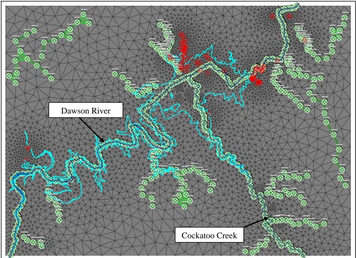
Figure 5 Rivers and drainage lines set in the Nathan Dam Groundwater Model
