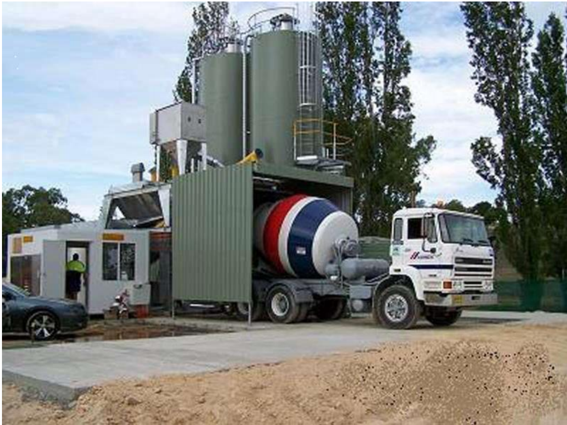
Figure 2-27 Typical mobile concrete batching plant
