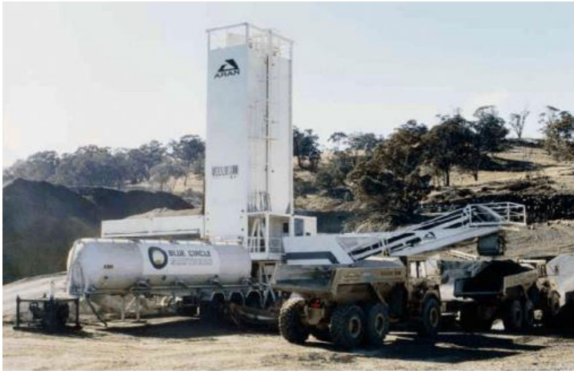
Figure 2-28 Typical mobile continuous concrete mixing plant
