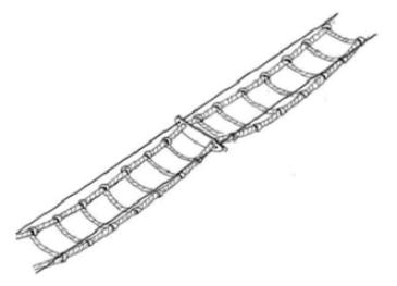
Figure 2.4 Rope ladder style canopy bridge overpass (from DTMR Design Manual Volume 2 (2010)
