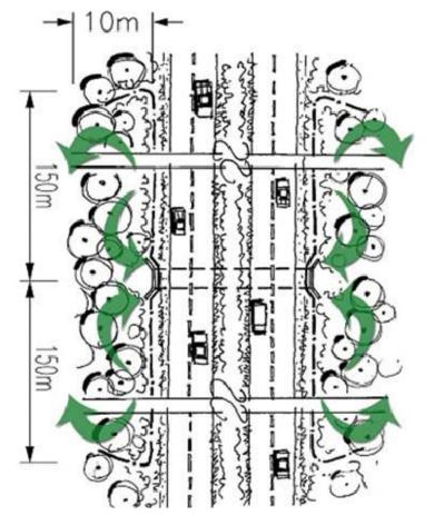
Figure 2.2 Optimal design of fauna exclusion fencing on either side of a crossing structure with incorporated returns at both ends (from DTMR Design Manual Volume 2 (2010))
