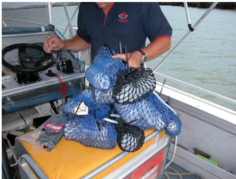
Figure 2. Deployment of the spiked seawater samples for field incubation in Port Curtis.
