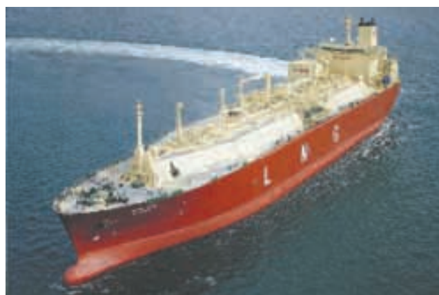
LNG tankers are double-hulled ships specially designed and insulated to prevent leakage or rupture in an accident.
