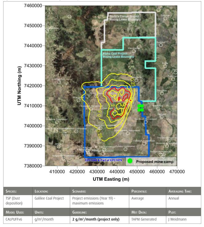
Figure 6: Predicted annual average dust deposition rates – Year 19 – maximum mine emissions
