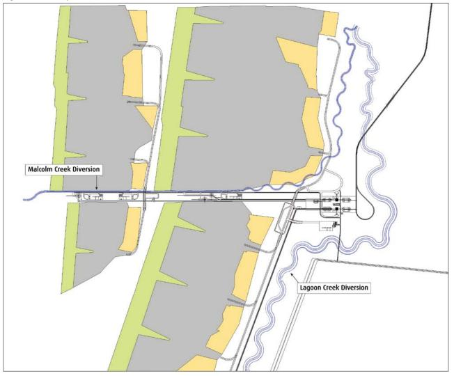
Figure 17: Concept of mine site creek diversions
