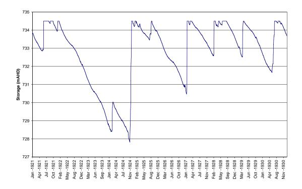
Figure 7 Dam water storage levels during a median period
