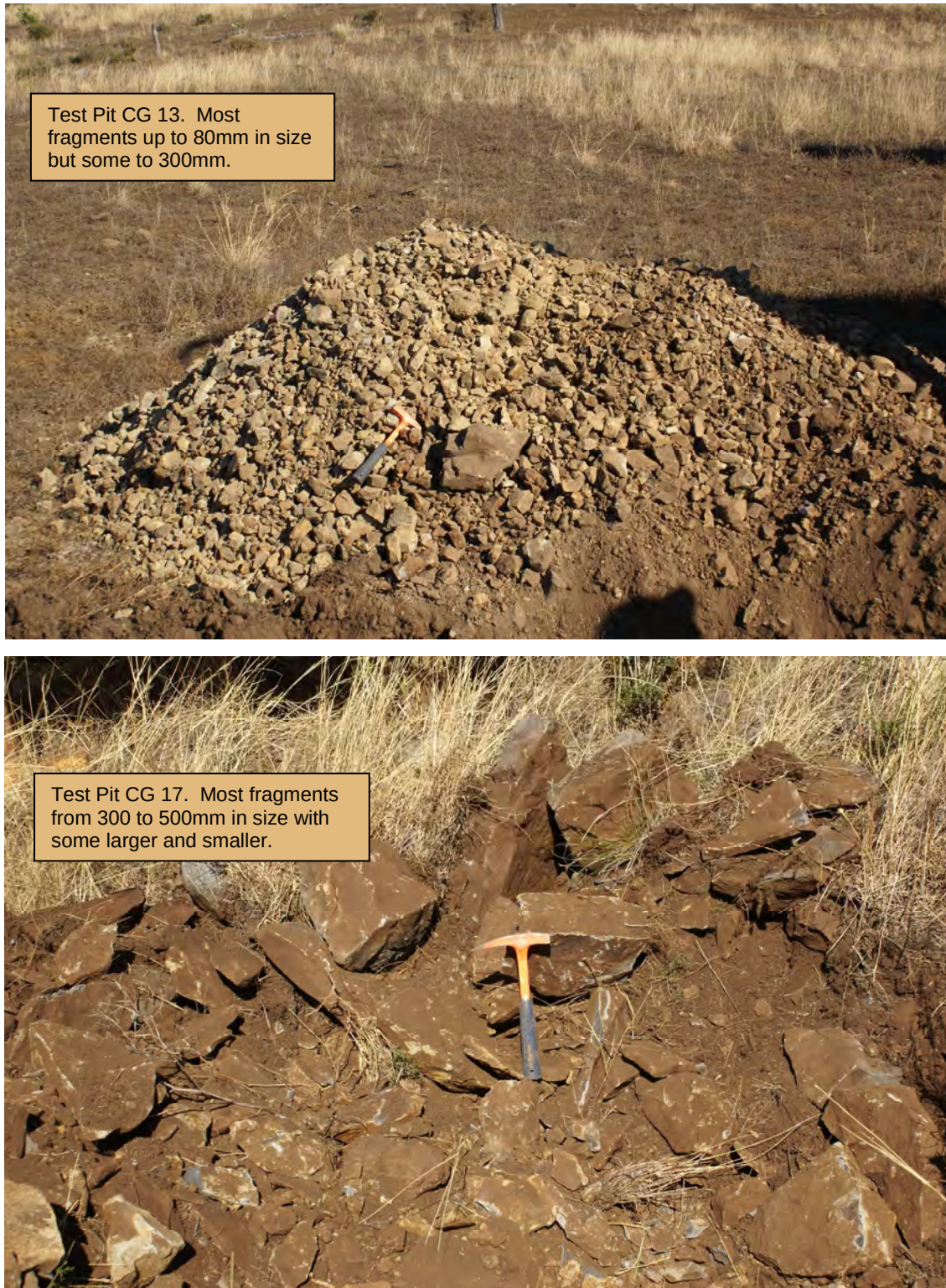
Figure 5.1. Comparison of Spoil from Two Test Pits
