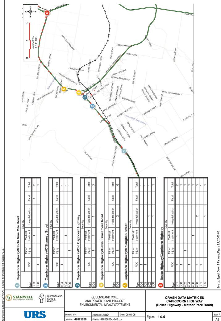
severity, and frequency is provided for locations recording high crash frequencies (i.e. more than three crashes).
