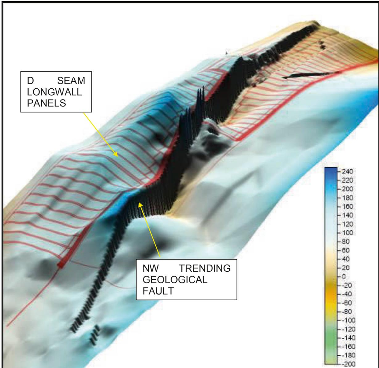
Figure 9. 3D Surface of the D Seam Structure Floor Levels (mASL).
