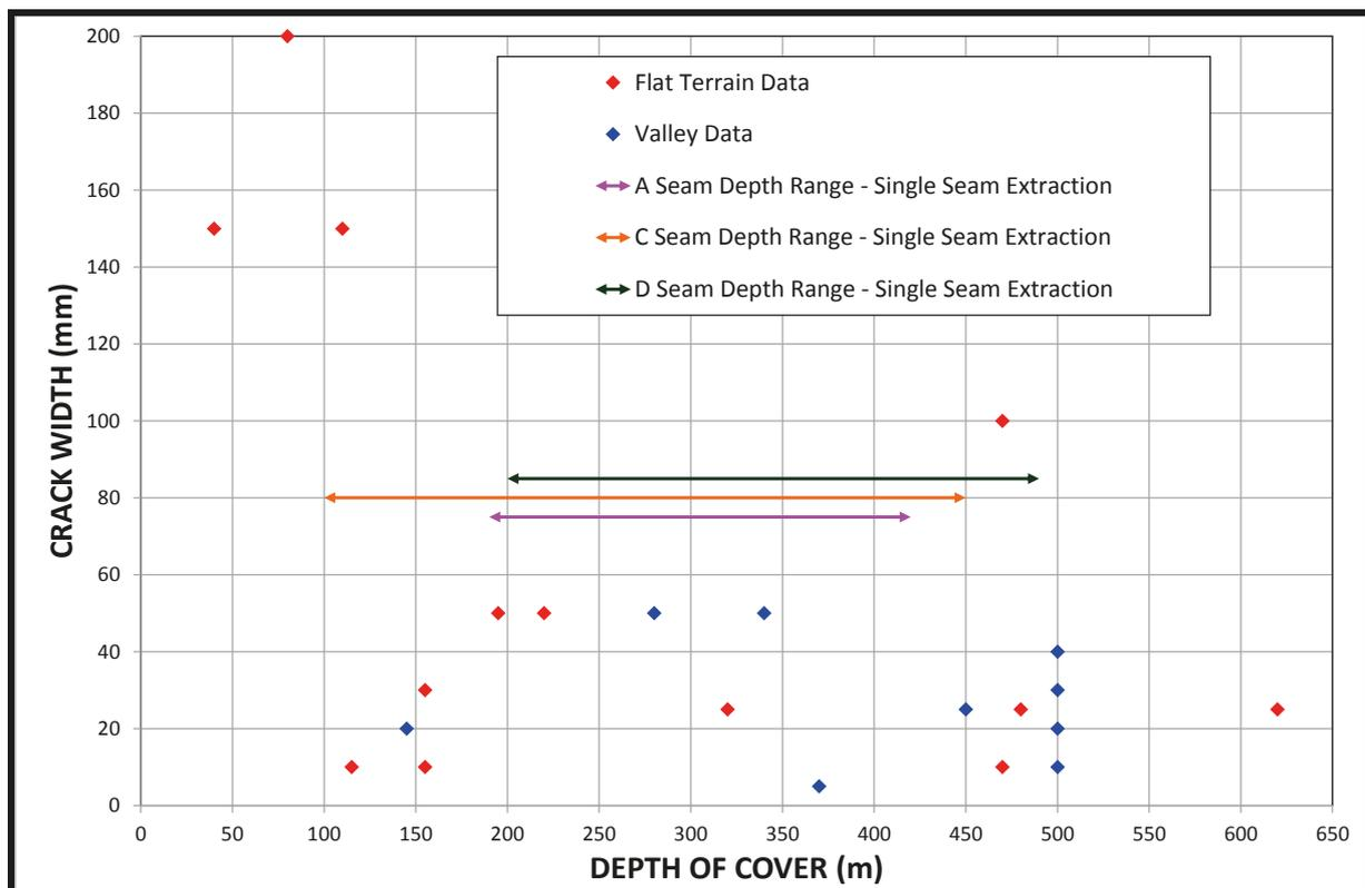
**Figure 38. Crack Width vs. Depth of Cover (reproduced from MSEC, 2007).**
