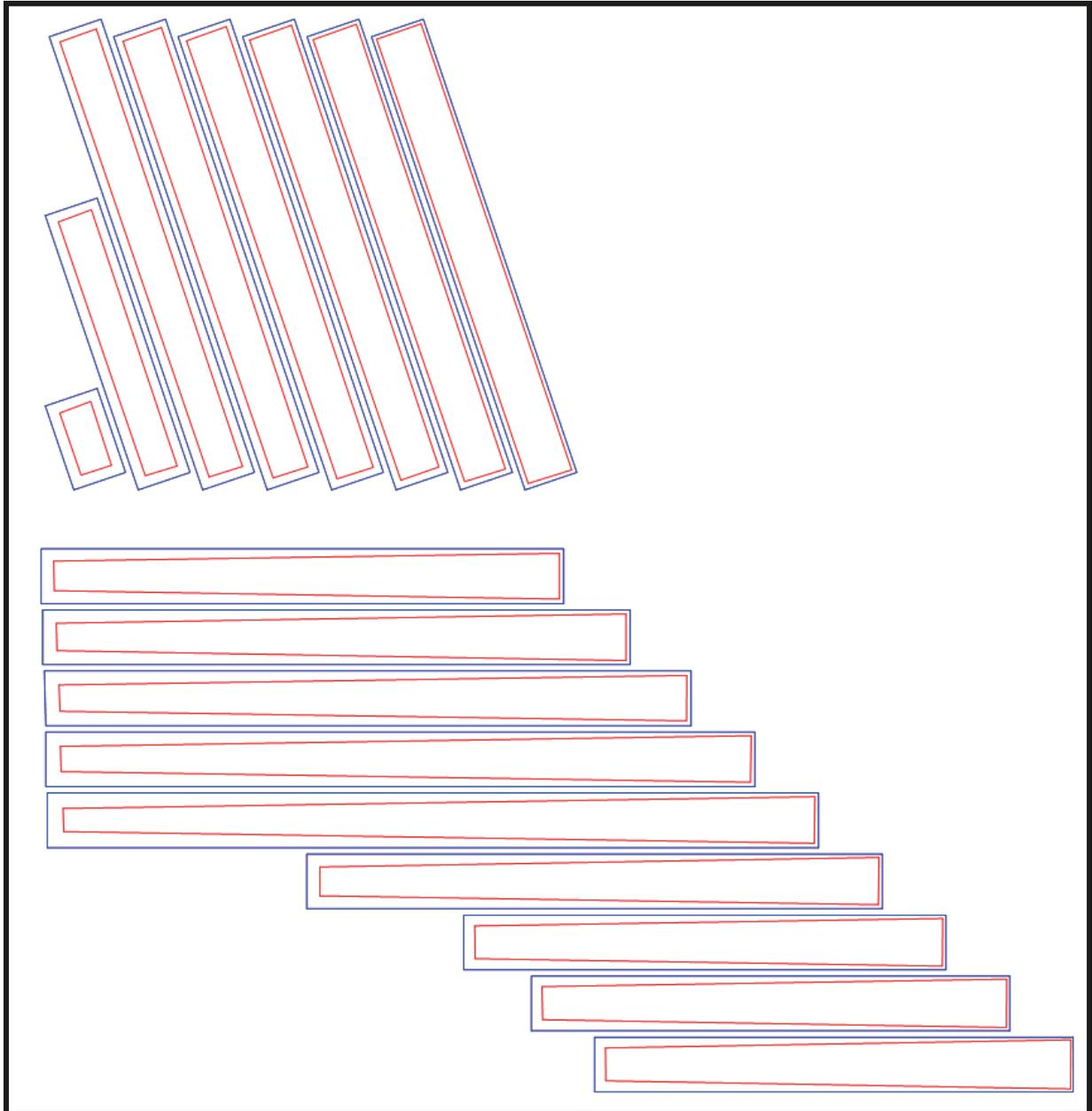
**Figure 14. C Seam Longwall Mine - Original Longwall Panels (blue) and Compensated Panels (red).**
