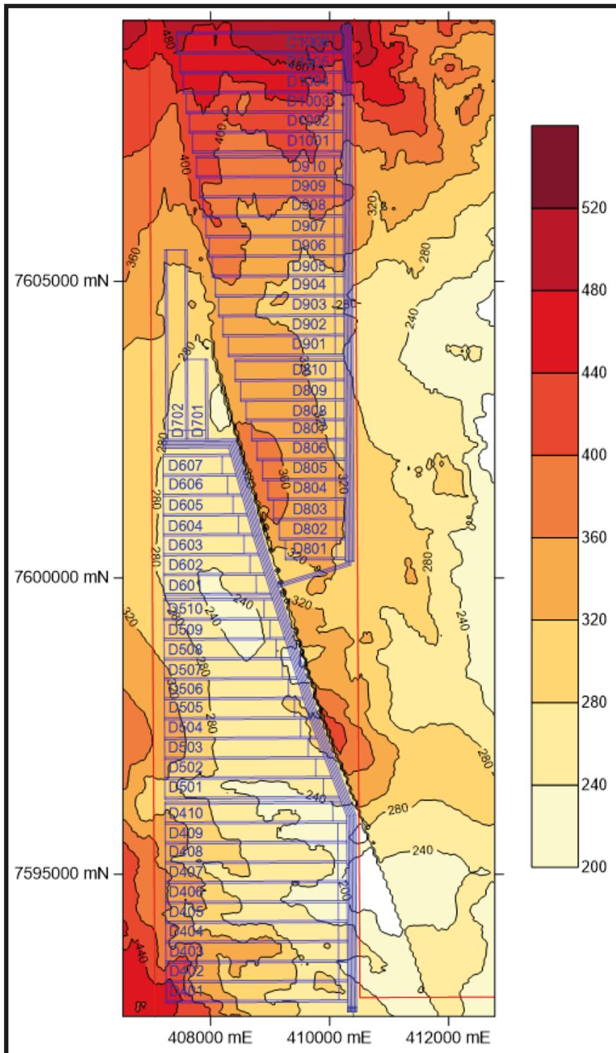
Figure 7. D Seam Depth of Cover (m).
