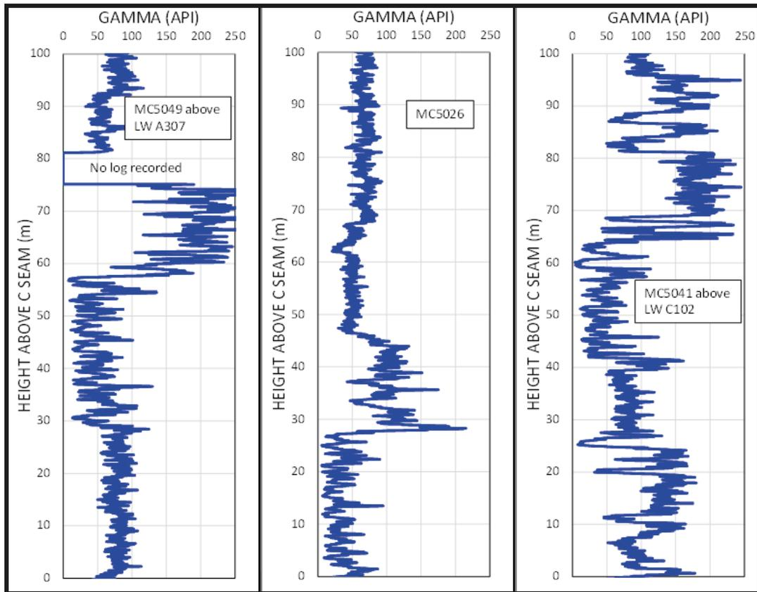
Figure 16. Gamma Response of the C Seam Overburden.
