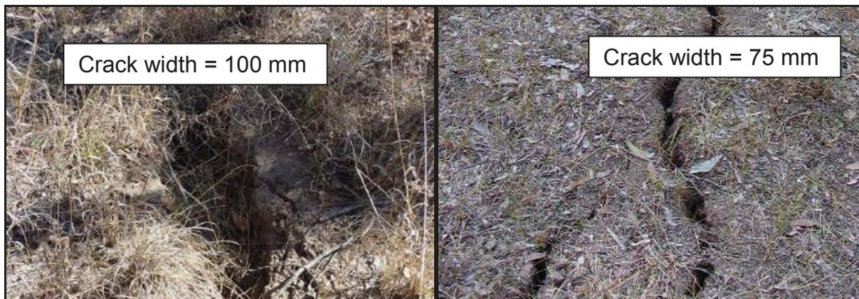
**Figure 39. Examples of Subsidence Cracks.**
