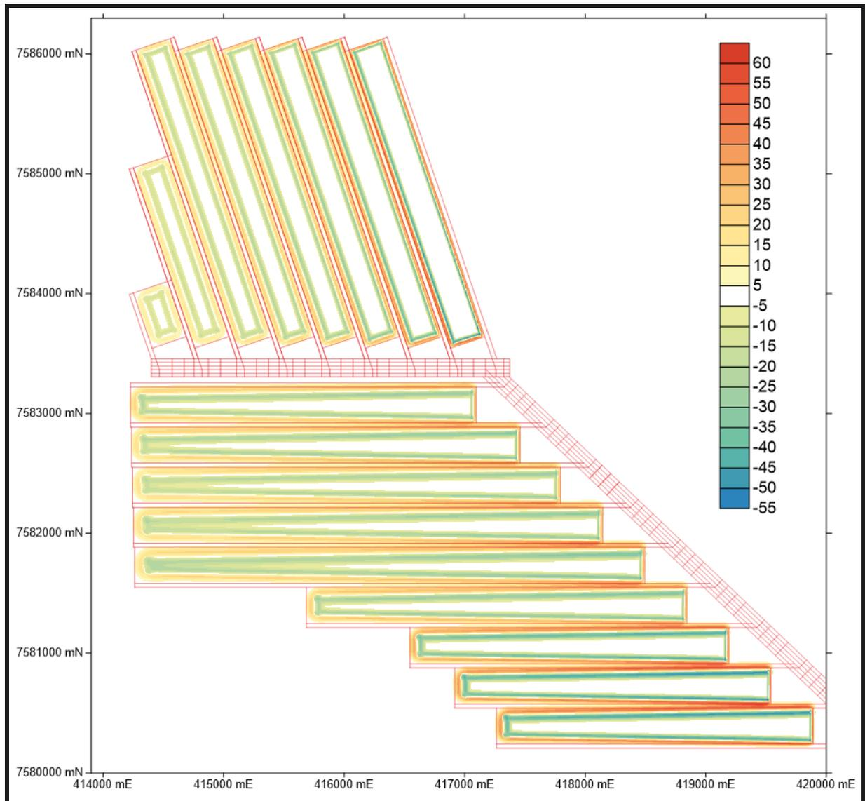
Figure 25. Strain due to C Seam Longwall Extraction (mm/m).
