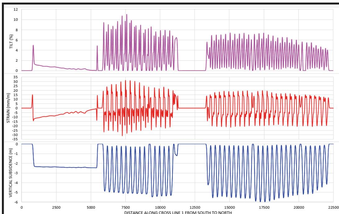
Figure 23. Subsidence, Strain and Tilt along Cross Line 1.
