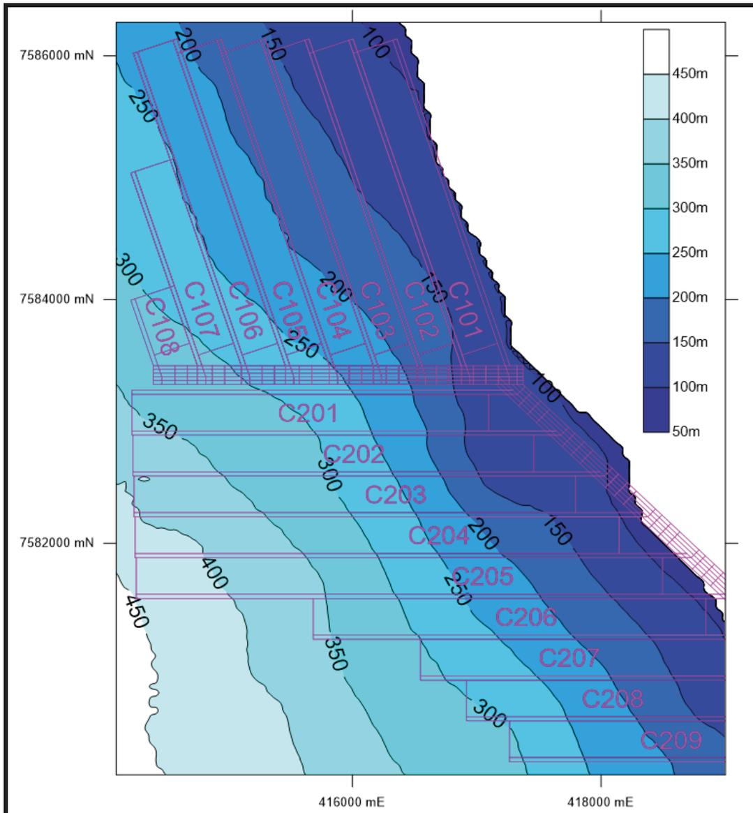
Figure 8. C Seam Depth of Cover (m).
