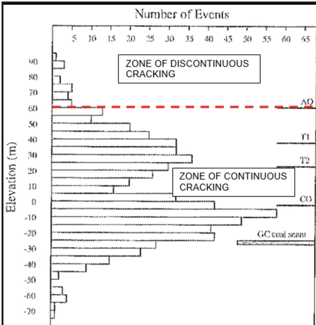
Figure 35. Location of Microseismic Events around LW101 at Kestrel Mine (Kelly and Gale, 1999<sup>11</sup>).
