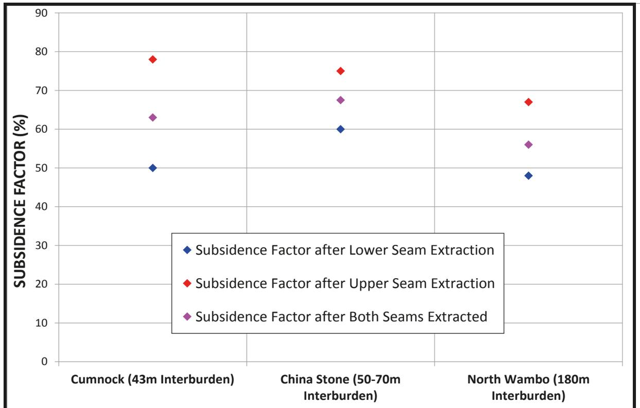
Figure 13. Subsidence Factors for Dual Seam Extraction.
