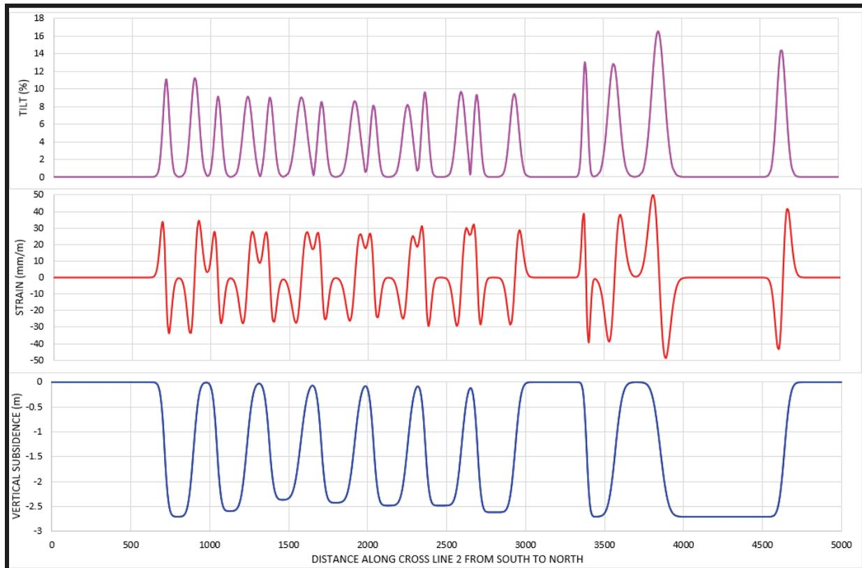
Figure 27. Subsidence, Strain and Tilt along Cross Line 2.
