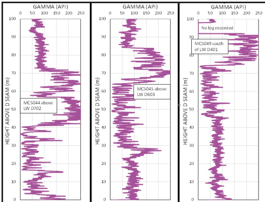
Figure 17. Gamma Response of the D Seam Overburden.
