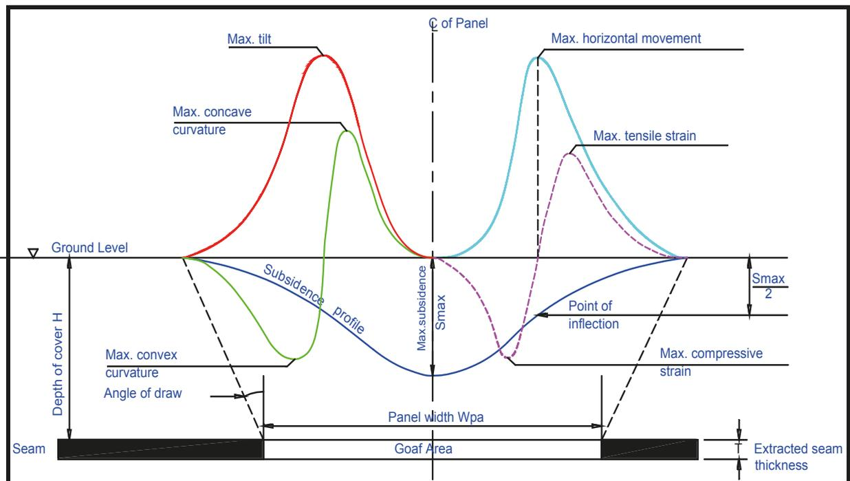
**Figure 11. General Characterisation of a Subsidence Cross Line.**
