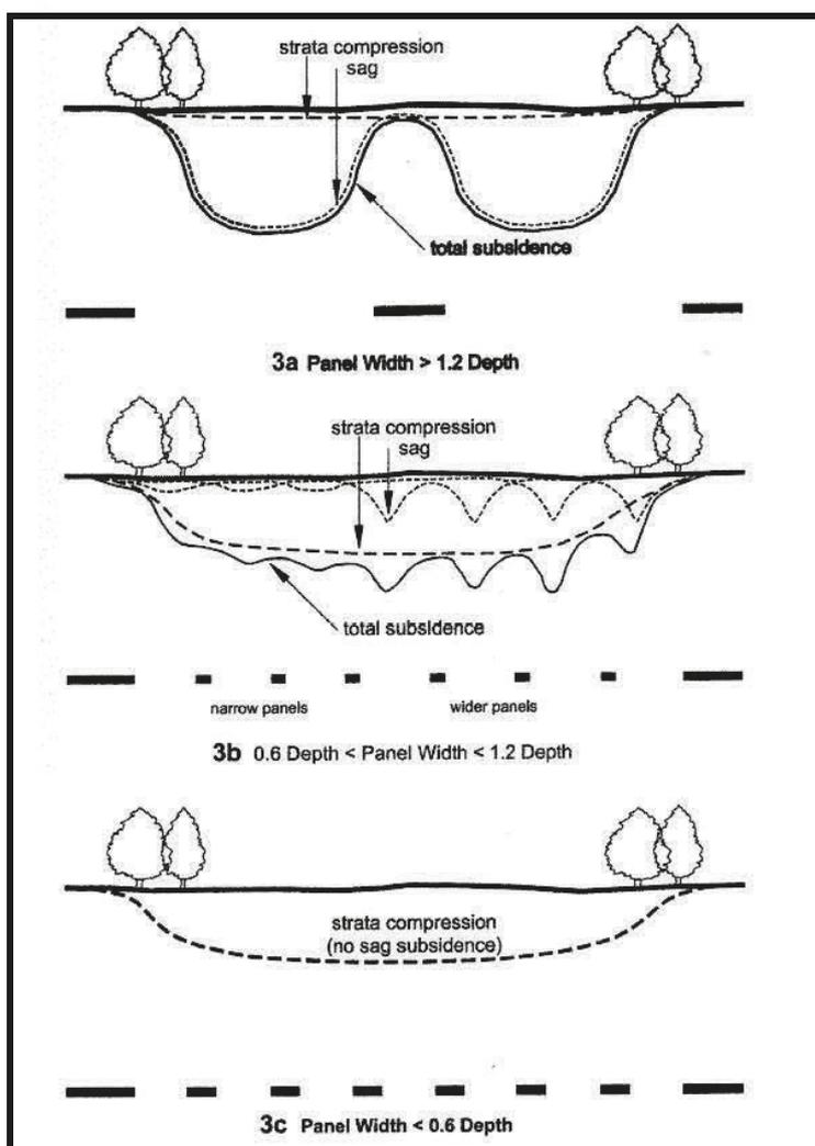
Figure 10. Effect of Panel Width (AusIMM, 2009<sup>4</sup>).
