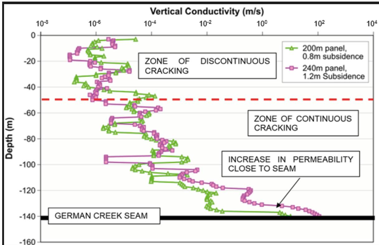
Figure 36. Vertical Conductivity through a Numerical Model in the Oaky Creek Mining Area (Gale, 2008<sup>12</sup>).
