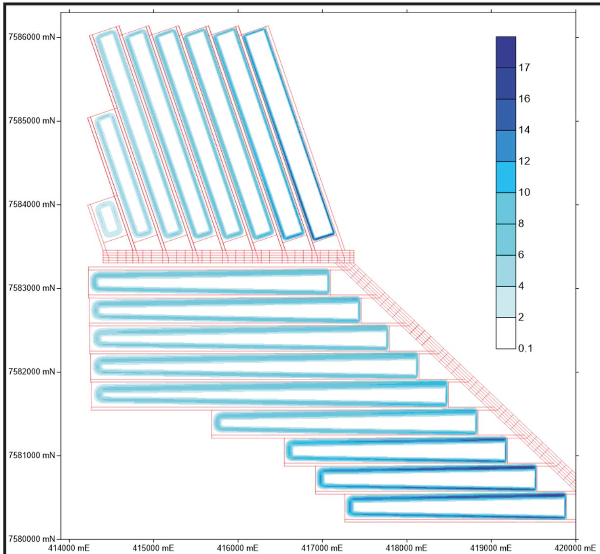
Figure 26. Tilt due to C Seam Longwall Extraction (%).
