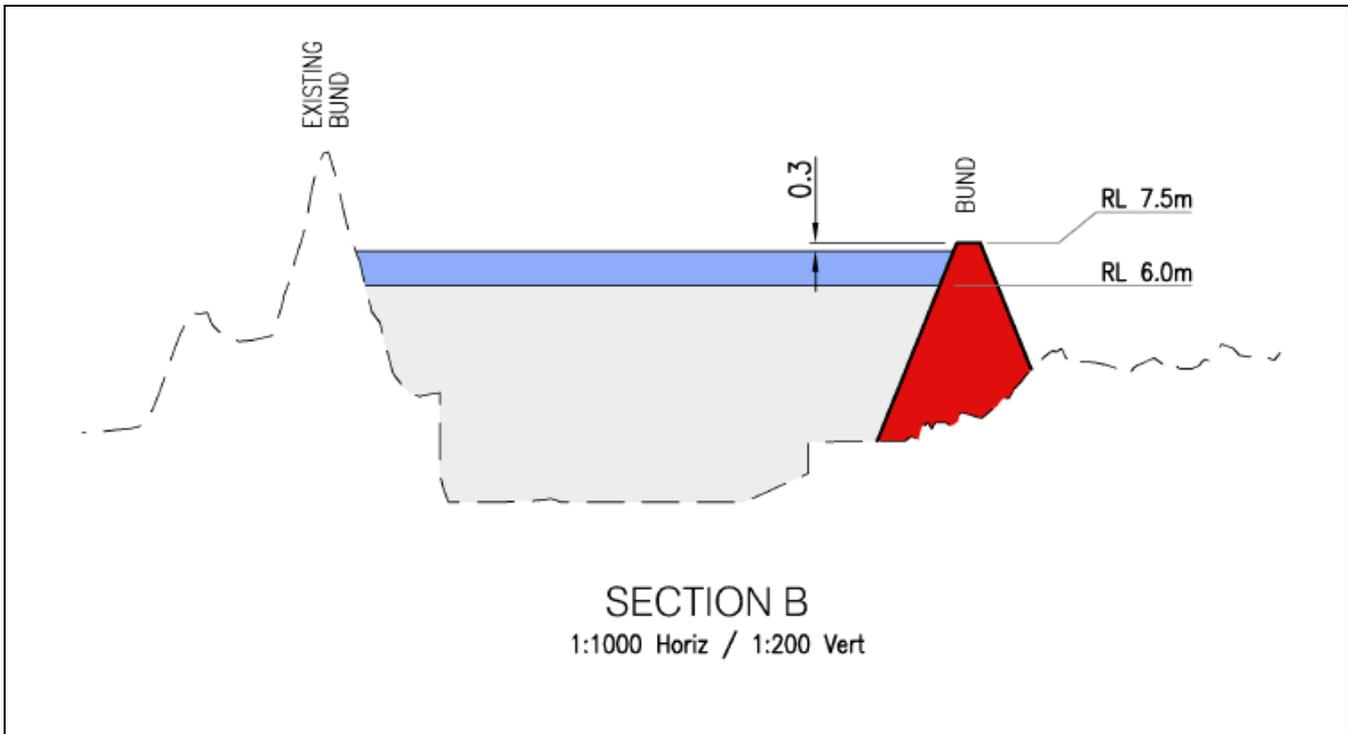
**Figure B17-11** Fill levels and water levels.
