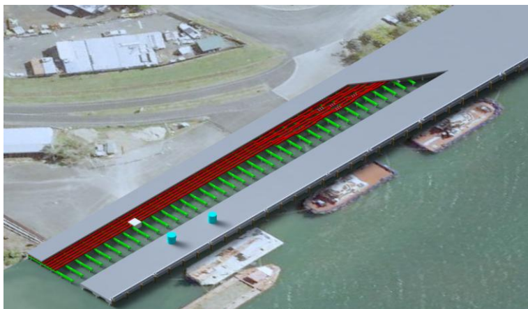
Figure 36. Option 2 – Detail of Wharf 5 & 6 interface area - Proposed treatment of the demolition of Wharf 6 and addition of extension to Wharf 5 at Cairns wharf (Ports North) – showing a small section of Wharf 6 retained along the foreshore, with exposed piles in the waterway between.
