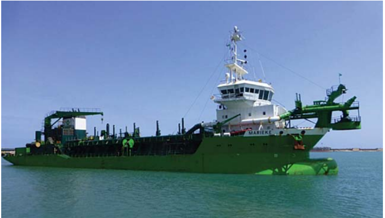
Figure C3.6.1b Example of a Medium Size TSHD
