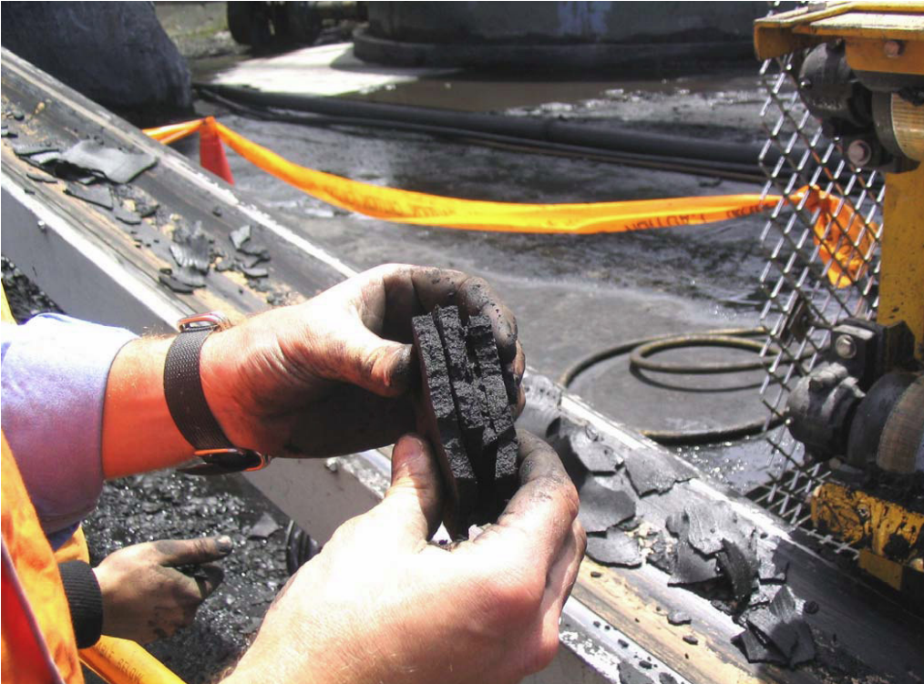
Figure 5 Final belt press filter cake prior to disposal
