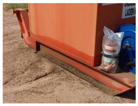
Plate 33 Staining on tank skids – Peak Downs Mine
