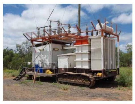
Plate 27 Mobile Dragline Transformer - Peak Downs Mine
