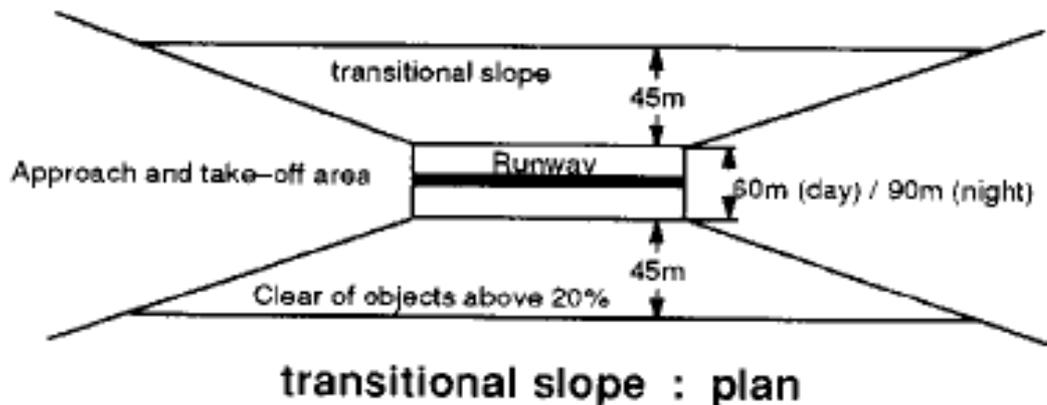
Figure 2.5 Dimensions for Night Operations (CAA1992)
