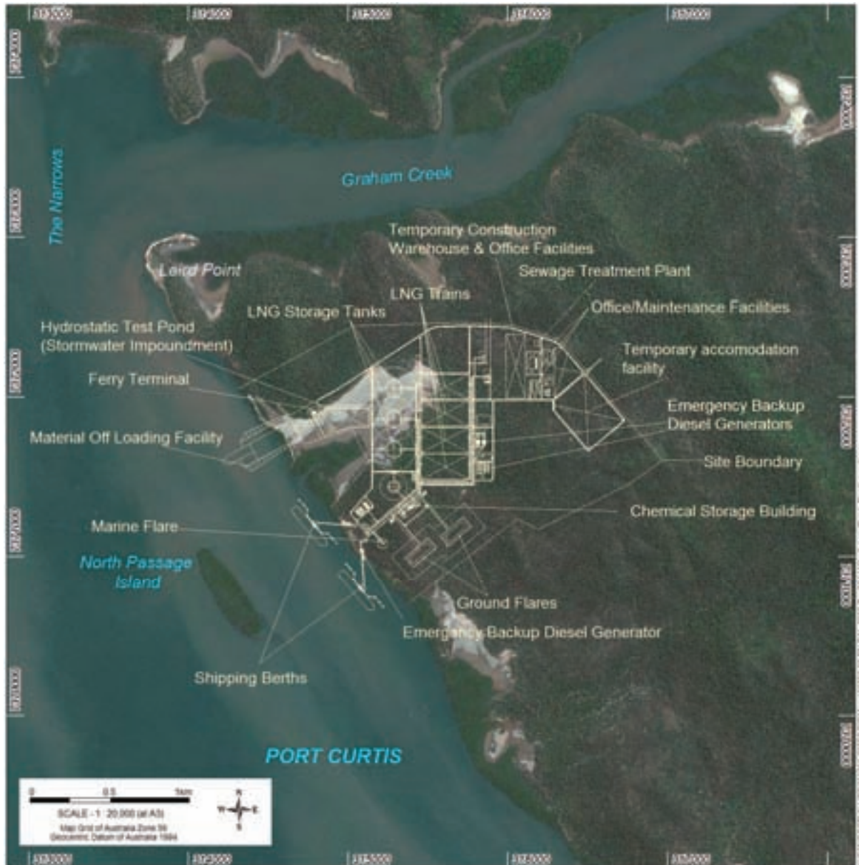
Figure 22.5 Indicative site plan for the LNG facility
